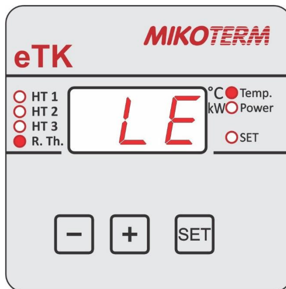
Image 23a: Temperature below -50^{\circ}\text{C} , or sensor short circuit
